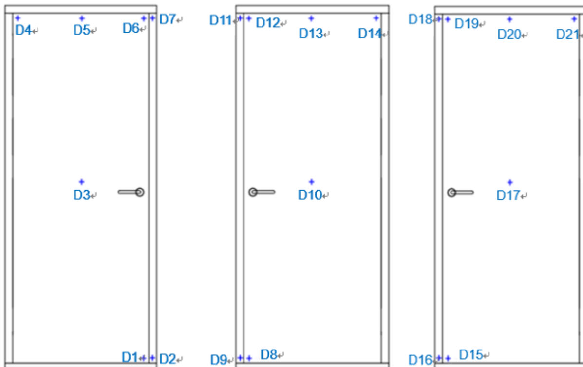
Figure 3 Positions for measuring horizontal deflection (View from unexposed side)
