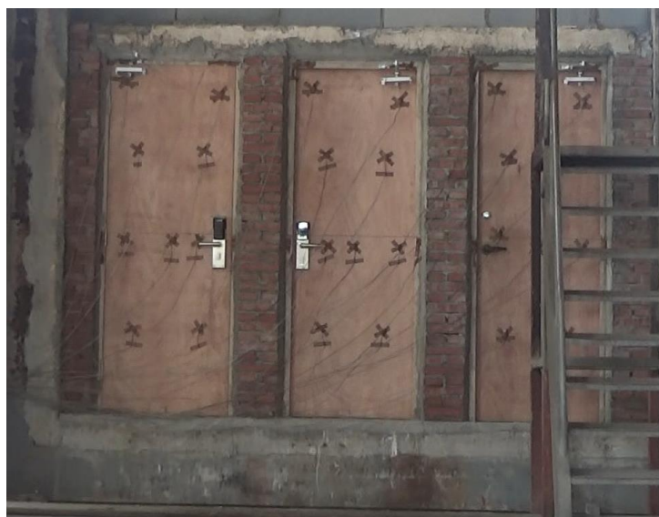
Unexposed face (Test before)
